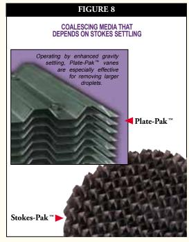
They make more efficient use of a vessel volume than a straight PPI (Parallel Plate Interceptor) since more metal is used and the specific surface area is greater. It can be shown from Equation 1 for  $V_t$  that the volume of media necessary to remove virtually all droplets equal to a minimum, typically 30-60 microns, is given by:
