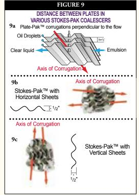
In order to decrease solid retention the axis of the corrugations of Plate-Pak should be parallel to the flow. However, vessel geometry often necessitates that the corrugations be perpendicular to the flow, especially in round vessels. Due to its light, self-supporting structure and ease of installation, the overall project cost is normally less for STOKES-PAK than Plate-Pak when
