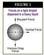
commonplace. In this equipment, differences in densities of the two liquids cause droplets to rise or fall by their buoyancy. The greater the difference in densities, the easier the separation becomes. Rising (or falling) droplets are slowed by frictional forces from viscous effects of the opposing liquid. When the stream is not
