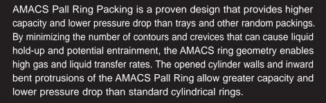
This open ring design also maintains an even distribution and resists wall-channeling tendencies. The interior and exterior contacting surfaces of the AMACS ring provide for an effective distribution of liquids and gasses and resist plugging, fouling and nesting. Pall rings are available from our stocked inventory in a wide range of materials.
