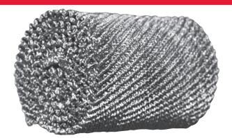
AKSP Tower packing is the AMACS Separation Products Goodloe® equivalent. AMACS high-efficiency structured packing is ideally suited for applications that demand high separation efficiency with a lower pressure drop. Its low HETP requirements result in smaller column heights.
